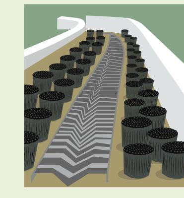
The fish pass is an innovative design by Dr Reinhard Hassinger from the University of Kassel, Germany. It's the first of its kind in the UK with the novel design combining concrete and naturalised sections, a resting pool and spawning grounds.
